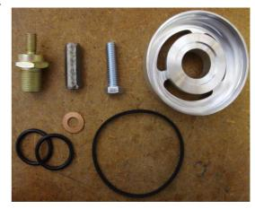
Remove the original filter bowl, filter and retaining bolt. Remove the old seal(s) from the filter housing. Fit the large square section seal in the outer groove of the housing. Fit one of the two o-rings into the groove in the centre of the housing.
